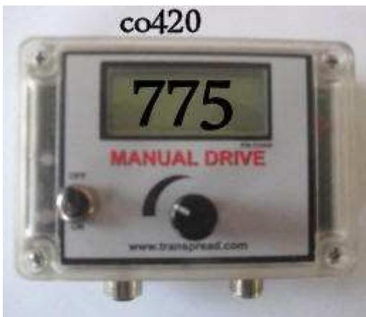
The control on the left will operate one spinner and give a readout of its speed. The operating speed is set by the computer and when this is fitted it will bypass some of the oil and slow the spinner down, the speed can be seen on the screen.
