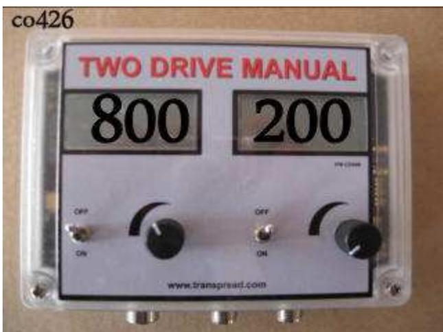
The one below will operate two spinners so you are not limited to one direction around a field.
